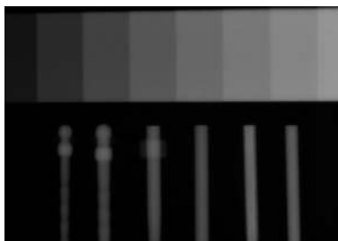
Figure 7.6 Aluminum step wedge from 1 mm to 8 mm thickness is used as reference for determining radiopacity of polymer based restorative materials (ISO International Standard 4049, 2009). X-ray shows radiopacity of prefabricated FRC root-canal posts (from the left: ParaPost Fibre Lux (Coltene/Whaledent); ParaPost Fibre White (Coltene/Whaledent); RelyX Fibre Post (3M Espe); Fibre Post (GC Corporation); Rebuilda Post (Voco); FRC Postec Plus (Ivoclar/Vivadent)).
